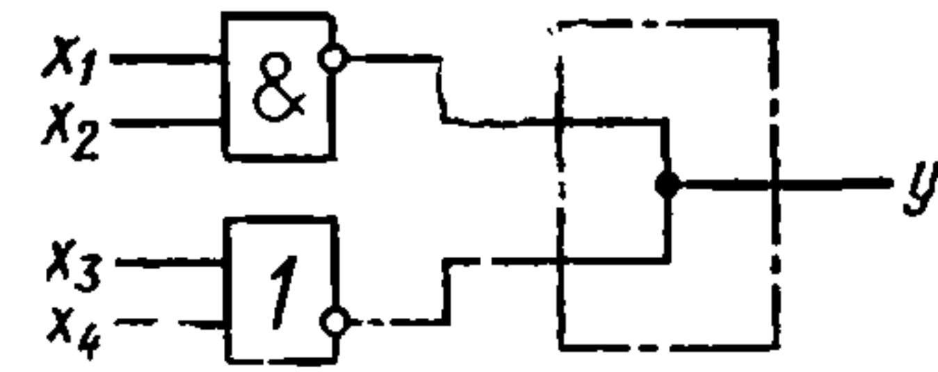
$y = \overline{x_1 x_2} + (\overline{x_3} + \overline{x_4})$ |
